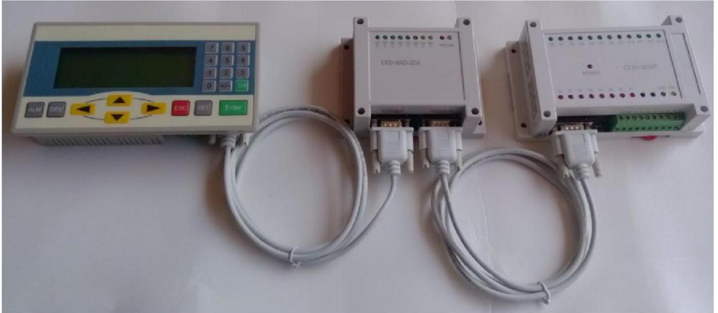
There are two communication ports above the module, one labeled "To PLC"
